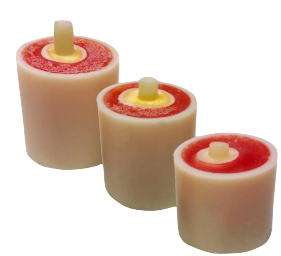
Figure 1 Shows the three subgroups of prepared specimen after composite build up. (6.0mm, 4.0mm and 2.0mm; left to right).
